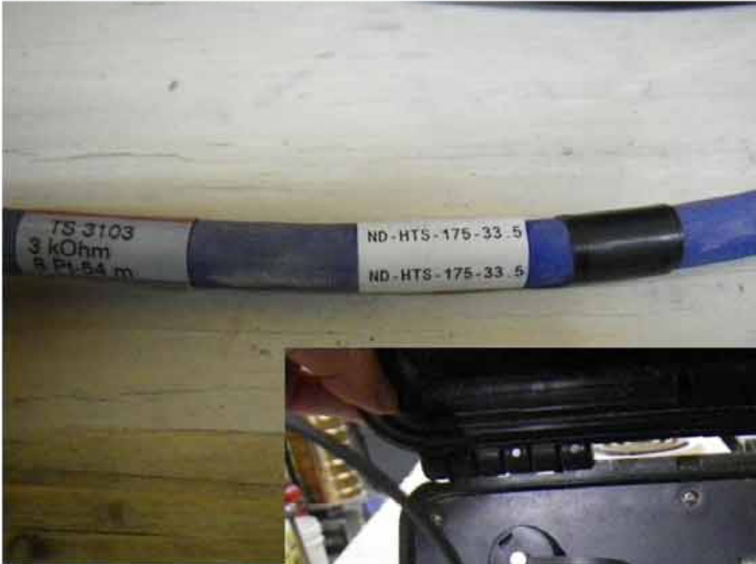
Photo 12 (above): Tape as secondary marker on ND-HTS-175-33.5 which is soon to be installed in the key trench.
